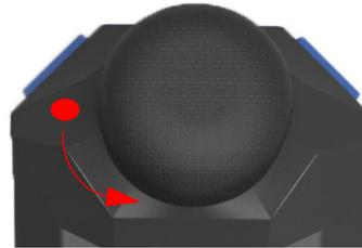
**Step 2.** Insert the microphone into the slot on the bottom of the calibrator. The adapter (ADP109) is required for a proper fit.
