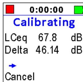
**Step 4.** When *Accept Cal?* appears on the dosimeter display, press **select**
