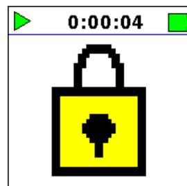
**Step 3.** Use the LD Atlas app or G4 to operate or unlock a locked dosimeter. For more information, in G4 go to **Help** → **Manuals** → **G4 LD Utility** → **6.1.3 Using the Meter Lock for Spartan 730 Dosimeter in G4**.
