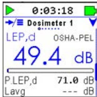
The Spartan 730 dosimeter configuration settings are displayed on the first 4 screens of the LCD. The LCD displays the current measurement data in terms of your chosen configuration for *Dosimeter 1*.
