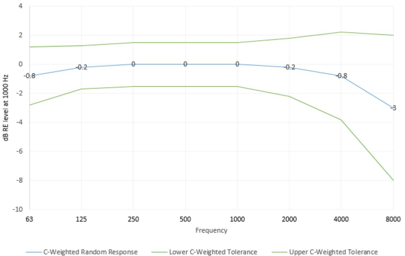
**FIGURE A-3 Model 730 RI Acoustic Response (Z-Weighted)**
