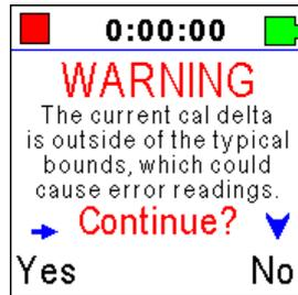
This screen notifies you that the dosimeter's current sensitivity is very different from the previously measured sensitivity. Changes like this indicate that it's time for your dosimeter to be serviced.
