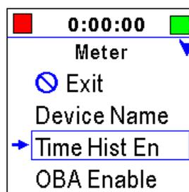
**Step 5.** Press **up** or **down** to toggle the option to **Enabled**.
