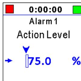
**Step 3.** Repeat the process shown in step 2 to set the **Limit Level** and return to the Alarm 1 menu.
