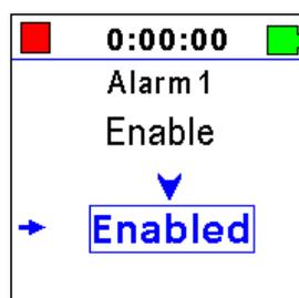
**Step 6.** Press **up** or **down** to toggle the option to **Enabled**.
