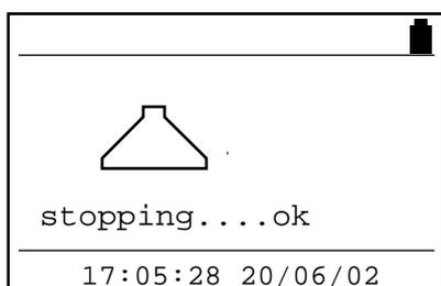
An indicator will flash through the doseBadge window to indicate the change from Run to Stop. Handling the doseBadge will now have no effect on the measurements and so the doseBadge can now be removed from the wearer.
