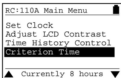
If the setting for the Criterion Time is not correct, the value can be selected from the list provided.
