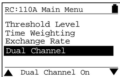
The options are to switch the Dual Channel Measurement On and Off.
