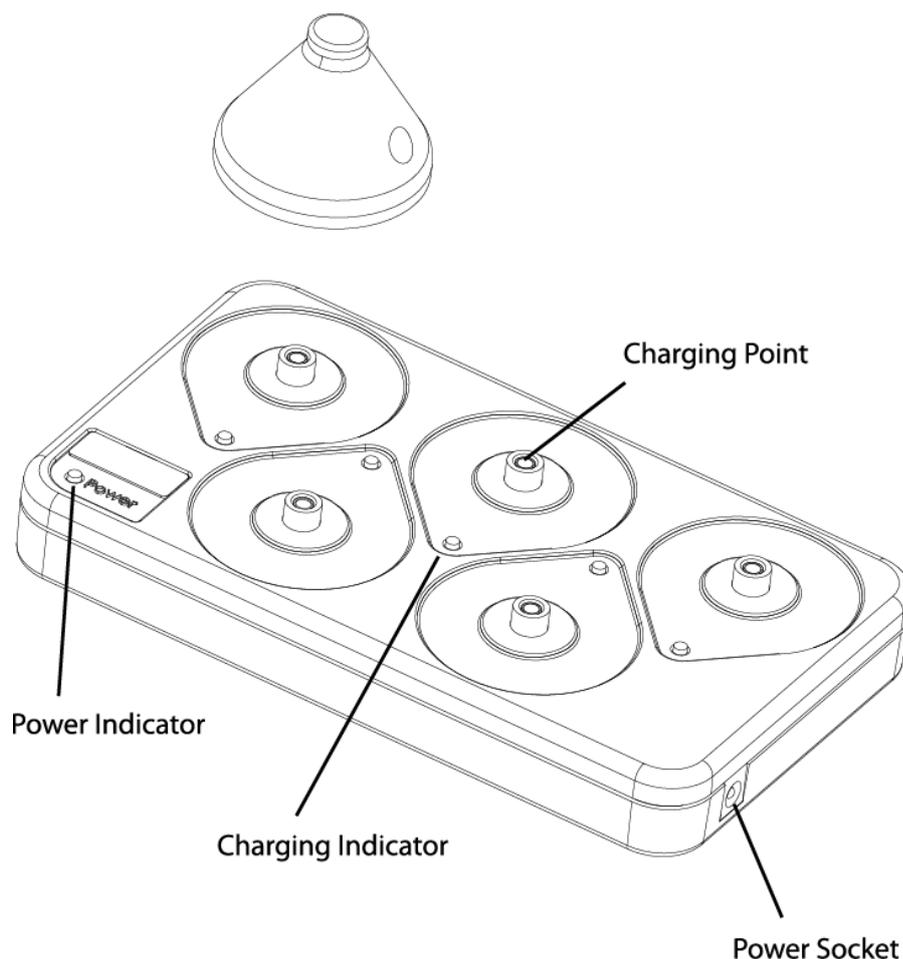
During the charge cycle, the green indicator will flash to show that the charging is in progress.
