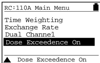
When this option is switched on, the LED indicator on the doseBadge will flash twice every second to indicate that the noise exposure has exceeded the 100% Dose value.
