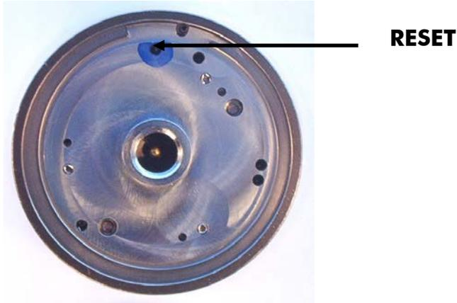
4. Move the metal object in the hole until you see the Blue LED flash through the optical window on the doseBadge. What you are trying to do with the metal object is connect the pin directly below the hole with the silver metal baseplate.
