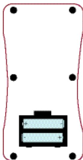
Remove the battery cover and replace the batteries.
