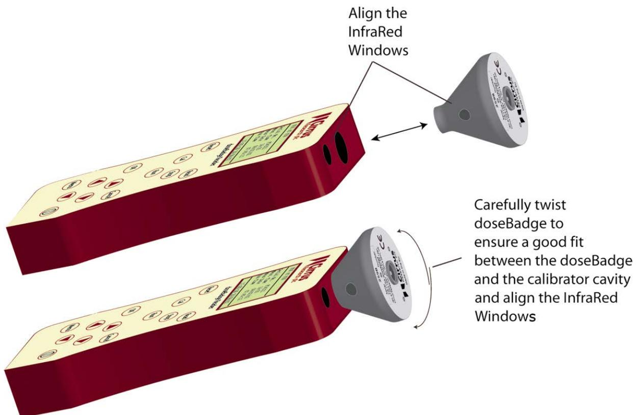
The doseBadge must be pushed firmly into the calibrator cavity to make sure that there is a good quality seal around the microphone. If the doseBadge is not pushed into the calibrator cavity, the acoustic calibration level will be reduced and the calibration will fail.
