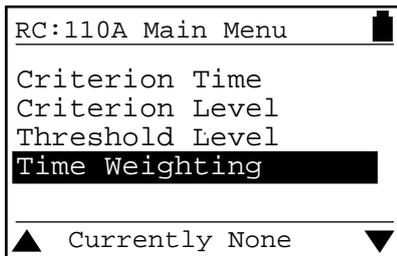
If the setting for the Time Weighting is not correct, the value can be selected from the list provided.
