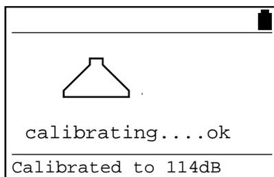
When the calibration is complete, the Reader unit will display the calibration information.
