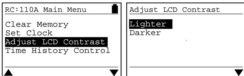
The contrast of the LCD display can be adjusted to accommodate different ambient light conditions. To change the contrast of the LCD display, press the OK key on
