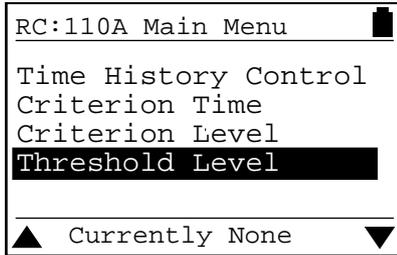
From the menu, select the Threshold Level position. The current setting for the Threshold Level is shown at the bottom of the screen. If the setting for the Threshold Level is not correct, the value can be selected from the list provided.
