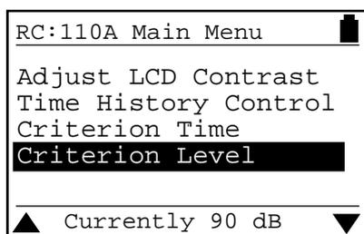
If the setting for the Criterion Level is not correct, the value can be selected from the list provided.
