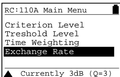
If the setting for the Exchange Rate is not correct, the value can be selected from the list provided.
